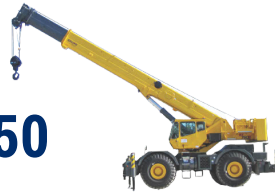
110 ft main boom and 33 ft - 56 ft bi-fold swingaway
